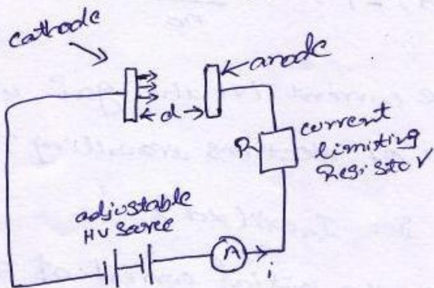
Let us assume that no electrons are emitted from the cathode. When one electron collides with a neutral particle, a positive ion and an electron are formed. This is called an ionizing collision.
