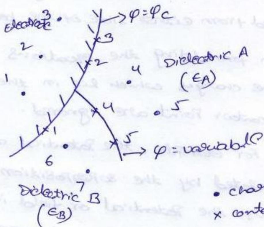
The field computations for a multi-dielectric system are more complicated than for a single dielectric. This is due to the fact that, under the influence of applied voltage, the dipoles are realigned in a dielectric, and this realignment has the effect of producing a net surface charge on the dielectric. Thus in addition to the electrodes, each dielectric-dielectric interface needs to be simulated by the discrete charges.
