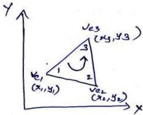
The above triangular element shows the potentials  $v_{e1}$ ,  $v_{e2}$  &  $v_{e3}$  at nodes 1, 2 & 3 are obtained from
