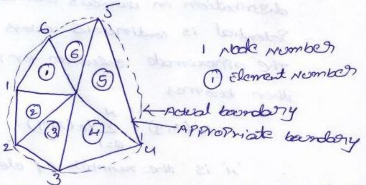
The potential, which is unknown throughout the problem domain, is approximated in each of these elements in terms of the potential at the vertices called nodes. As a result of this the potential functions will be unknown only at nodes. Normally a certain class of polynomials, is used for the
